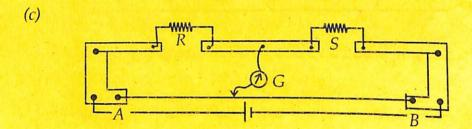
In the meter bridge shown in the above figure, the null point is found at a distance 33.7cm from A and of the wire for particular values of R and S. If a resistance of  $12\Omega$  is connected parallel with S, the null point is found to be at 48.1cm from B end. Determine the value of R and S.
